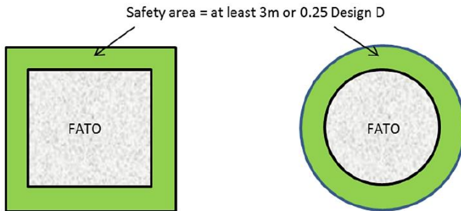
Figure 3-1. FATO and associated safety area
